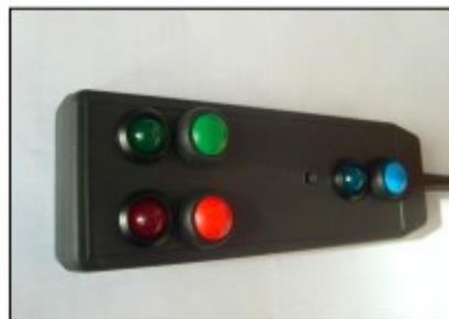
PRESSING the **GREEN BUTTON** means that there is NO NEED to send the emergency service (OK).
