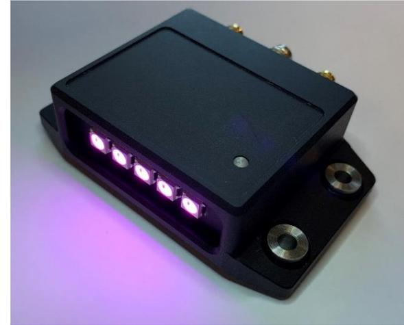
Fit the Racelink on your (clean) dashboard, and make sure the driver can see the LED's on the front of the Racelink. Additional/alternative installation tips are shared via the Sportity app.
