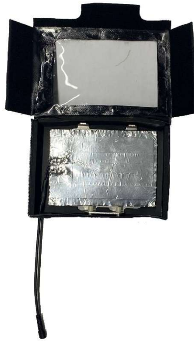
Fig. 10 The heating plate installation.
