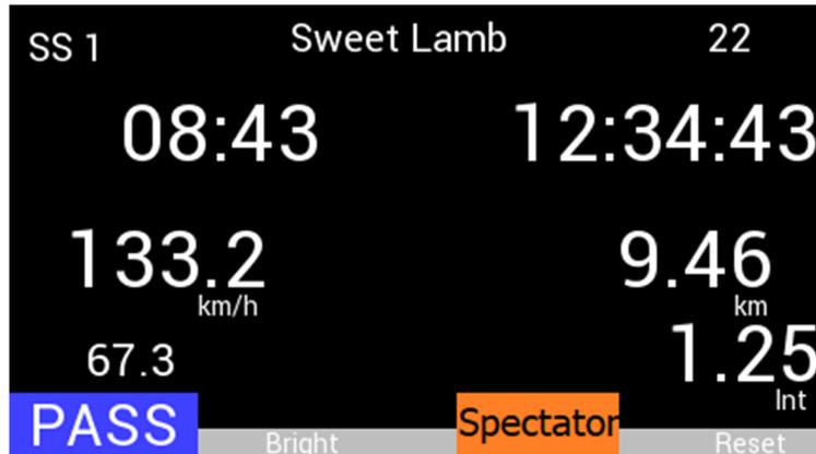
At the request of Motorsport Australia, a modification has been made to the RallySafe Unit, to enable competitors to inform Race Control of the location of “Dangerous Spectators”.
