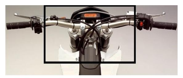
Additional compulsory requirement for class B only: TWO lights (like LED repeaters) must be visible from 10 meters away positioned on the both sides of the motorcycle (located in the identified area, please see the diagram hereunder). These two sides indicators must be protected from any possible contact (rider, environment, etc.).
