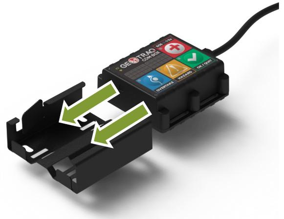
**IMPORTANT! THE ANTENNA NEEDS AT LEAST 55mm ON ALL SIDES TO WORK PROPERLY! MAKE SURE NOT TO PLACE IT RIGHT NEXT TO OTHER METAL COMPONENTS!**
