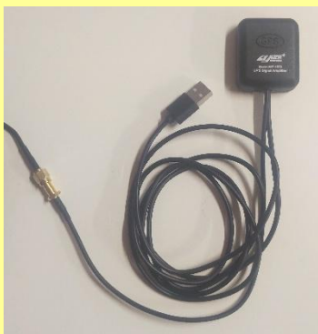
Inner antenna with usb-connector for power supply 5V (USB Cable approx. 1 metre long
