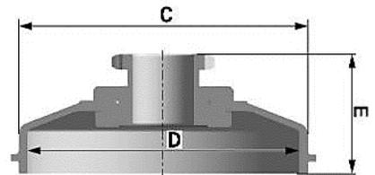
Clutch drum Inner diameter (D):
