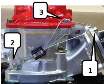
By means of the steel cable the engine must be sealed on one allen screw of the intake flange (1), one stud screw of cylinder (2) and one allen screw of the cylinder head cover (3) - see left picture.
