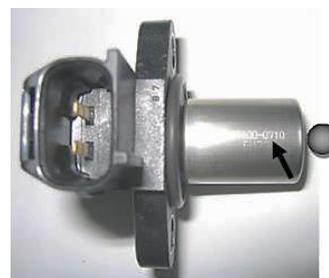
Mounting the pick-up to the crankcase with a gasket additional to the original rubber sealing ring of the pick-up, is a legal specification.
