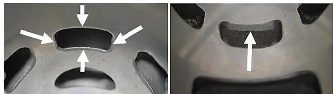
5.5.2.3 The flange for the exhaust socket may show either cast finish or machined surface. Machined surface can be either flat or show a circular sealing bump.
