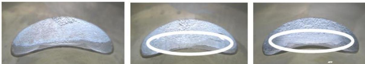
The exhaust port may show partial manual grinding done by the manufacturer to eliminate minor casting defects and/or to eliminate the NIKASIL burr at the end of the NIKASIL plating (see above right picture).
