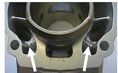
5.5.2.2 All ports have chamfered edges. Any additional machining is not permitted.
