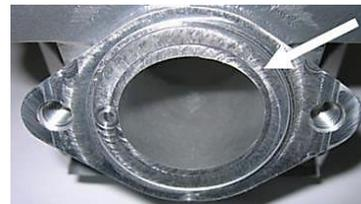
5.5.2.4 The top edge of the exhaust port may show either just a cast finish surface (left picture) or signs of a CNC machining (central picture) or signs of CNC machining in combination with signs of manual grinding (right picture).
