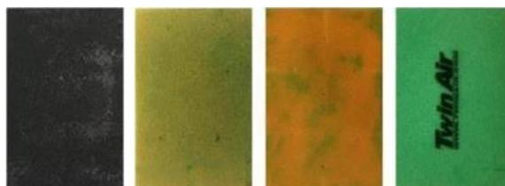
Depending on the degree of oil-lubrication colours may alter slightly or the surface becomes stained (see examples).
