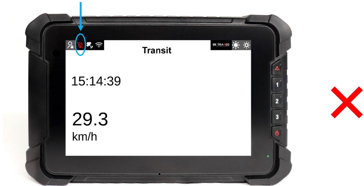
Figure 2 - Red power indicator light: device not powered
