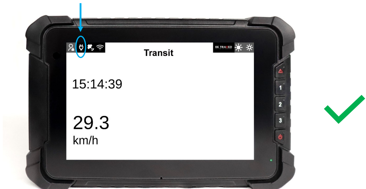
Figure 1 - White power light: device powered correctly
