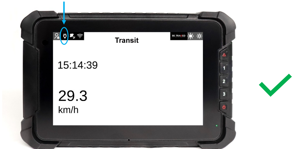
Figure 1 - White power light: device powered correctly
