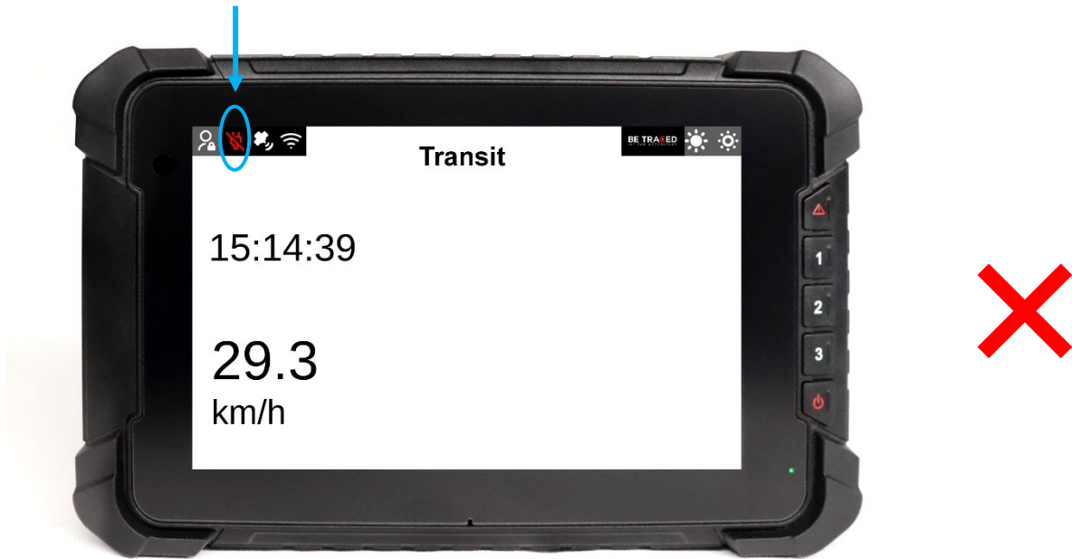
Figure 2 - Red power indicator light: device not powered
