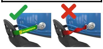
Ensure that the tethers attached to the harness and helmet without twisting.
