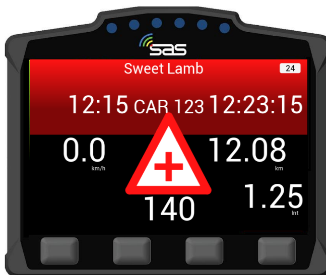
SCREEN 12. SOS proximity warning
