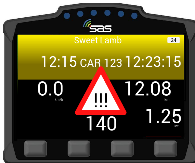
SCREEN 11. HAZARD proximity warning
