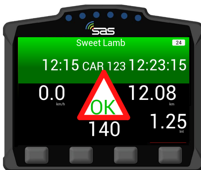
SCREEN 10. OK proximity warning
