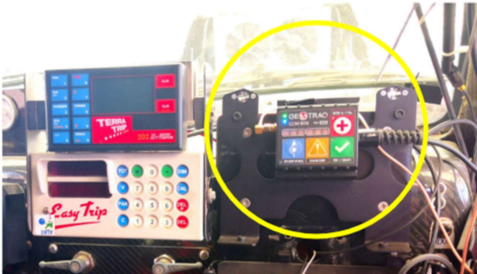
Installation of the Com-Box unit with bracket on the dashboard using bolts. This must be in a CENTRAL location and not as indicated above, only in front of the co-driver.
