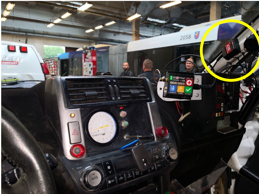
Installation of the GPS TRACKER on the roll cage “A-pillar” of a Car using cable ties.
