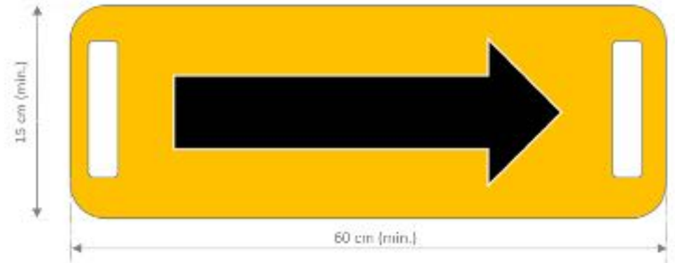
SIDE 1 - USING TOGETHER WITH THE YELLOW FLAG TO INDICATE THE SAFEST DIRECTION TO PASS THE OBSTACLE.
