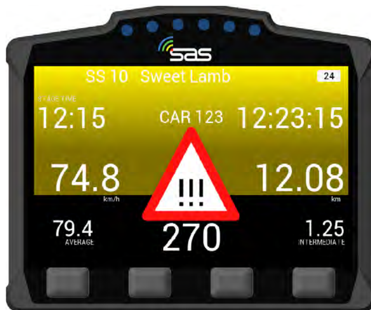
SCREEN 21: Hazard – Vehicle is on / next to the road – Status not confirmed [HAZARD]
