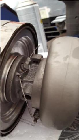
*Examples of incorrect sealing wiring*
