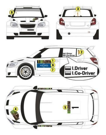
**DOOR PANELS (1)** - Each panel with 67cm wide and 17cm high shall be placed horizontally at the leading edge of each front door with the number at the front. The top of the panel shall be between 7 cm and 10 cm below the lower limit of the window. The remainder of this door panel is reserved for mandatory advertising of the organiser.
