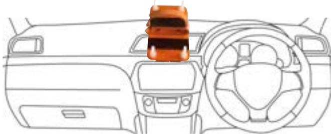
The device must be fitted in the centre of the dashboard accessible to both Driver and Co-Driver.
