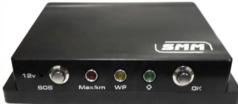
**Indicator «12v»** - indicator for turning on the device.
