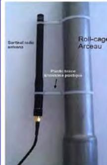
Fig. 6. Antenna mounting
