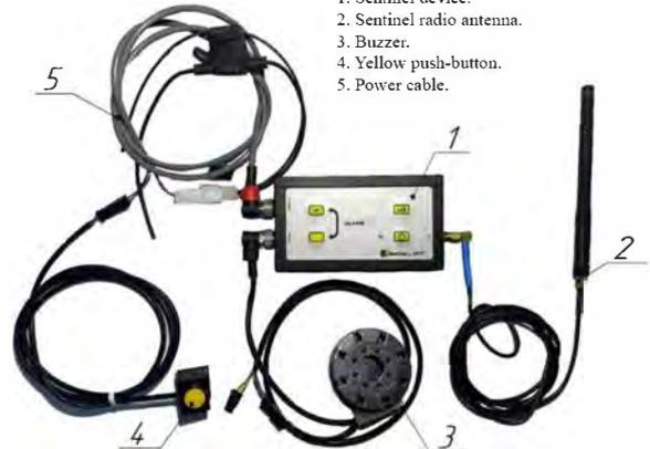
Fig. 5. Sentinel system kit assembled
