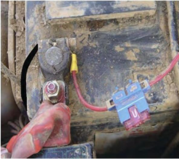
Connect the red wire to +12V (red terminal), and the black wire to the negative terminal of the battery.
